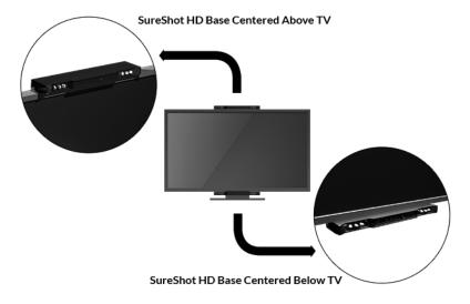
4. Make sure the Sure Shot HD Base is level with the ground and centered either directly above or below the TV, with the LED lights facing forward.
