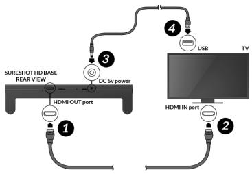
7. If you **do not** have a USB port on the back of your TV, plug the circular end of DC 5v power cable into the circular DC 5v port of your Sure Shot HD Base, plug the other end into a USB AC Adapter (not included), and plug the adapter into the wall outlet.
