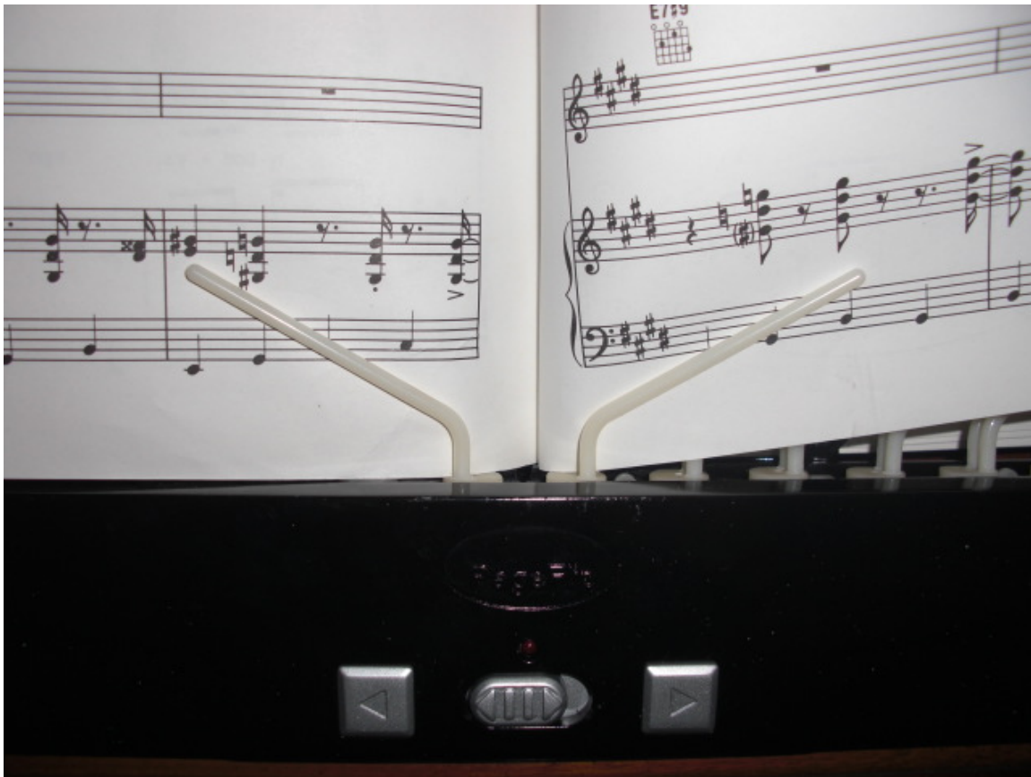
Figure 8: Pages in arm slots are restrained until they are turned one at a time.
