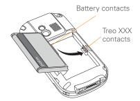
**IMPORTANT** Use the battery that came with your Treo XXX. Do *not* use a battery from another Treo model in your Treo XXX. Similarly, do *not* use the Treo XXX battery in another Treo model. Using a battery that is designed for another Treo model can damage your Treo XXX.
