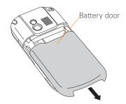
**3** Place a finger in the notch next to the battery, and lift up the old battery at a 45-degree angle to remove it from the compartment.
