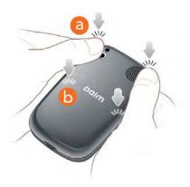
**10**Slide out the keyboard (see <u>Slide out the keyboard</u>), and then press the two snaps at the bottom corners.
