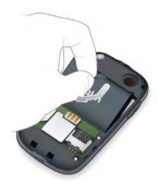
**WARNING** You must remove the battery first whenever you insert or remove the SIM card.
