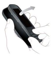
Remove the **battery** by putting your finger in the recess to the right of the battery; push the battery left and then lift it up and out.
