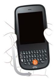
7 Swing the body of the phone out of the back cover as if the right side were a hinge.
