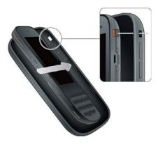
12 Press the back cover and the body of the phone together at each pair of clasps. You can feel the clasps engage.
