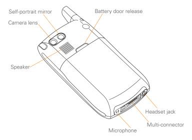
**IMPORTANT** The Treo smartphone speaker includes a large magnet, so be sure to keep your smartphone away from credit cards or other items that could be demagnetized.
