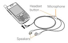
When using the headset that is included with your smartphone, you can press the headset button to perform any of the following tasks:
