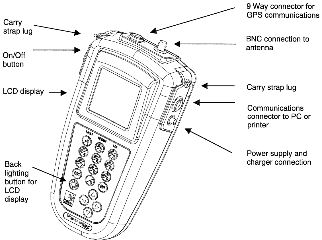
Patroller unit: connections and interfaces
