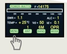
Press and hold the < or > arrows to increase or decrease ALC BASE VALUE. If using ALC this should be adjusted carefully to match your transceiver's requirements (usually -1.5V approximately).
