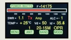
NOTE: Wattmeter only shows RED power bar graphical indicator when the LA-1K is transmitting.
