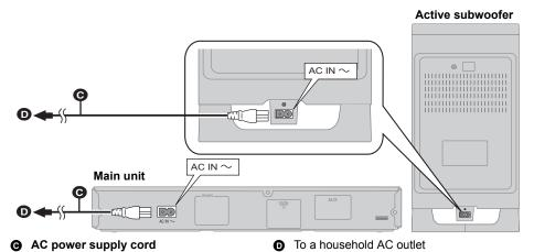
●The main unit and active subwoofer consume a small amount of AC power, even when it is turned off (this unit: approx. 0.1 W, active subwoofer: approx. 0.1 W). In the interest of power conservation, if you will not be using this system for a long time, unplug it from the household AC outlet.
