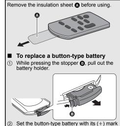
Set the button-type battery with its (+) mark facing upward and then put the battery holder back in place.
