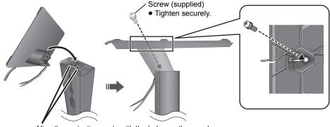
Align the projecting parts with the holes on the speaker.
