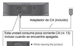
unused for a long time, turn off the unit and pull the AC adapter
