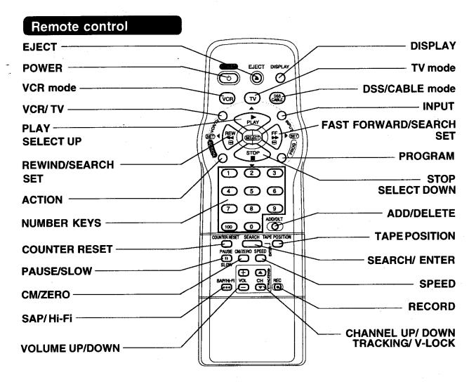
**EJECT button:** Press to eject tape from VCR. If EJECT is pressed during record, VCR will not respond.
