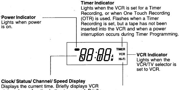
Displays the current time. Briefly displays VCR status when a function button is pressed. Briefly displays the channel number, or "L1" or "L2" when a channel or line input is selected. Briefly displays the recording speed when SPEED is pressed.
