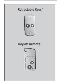
Use the keys to start and stop the engine, and to lock and unlock all the doors and tailgate. You can also use the remote transmitter to lock and unlock all the doors and tailgate.
