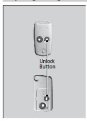
**To open:** Press the UNLOCK button twice within 10 seconds and hold it down for the second time.
