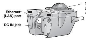
**Tripod Mounting Hole**Used when installing the camera on a tripod.
