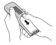
2 Insert the batteries negative (⊝) end first. Close the handset cover.
