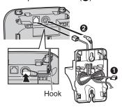
Insert the hooks on the wall mounting adaptor into holes (A) and (B) on the base unit.
