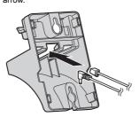
Tuck the telephone line cord inside the wall mounting adaptor (♠). Connect the AC adaptor cord and telephone line cord (♠).
