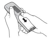
2 Insert the batteries negative (⊝) end first. Close the handset cover.
