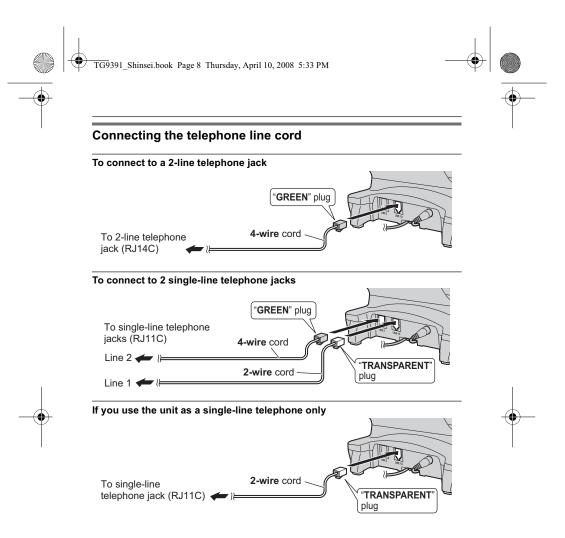
L Use only the supplied telephone line cord. Using another telephone line cord may not allow the unit to work properly.
