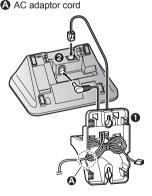
3 Insert the hooks on the wall mounting adaptor into holes (((a)) and ((b)) on the base unit.
