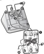
Insert the hooks on the wall mounting adaptor into holes (**(A)**) and (**(B)**) on the base unit.
