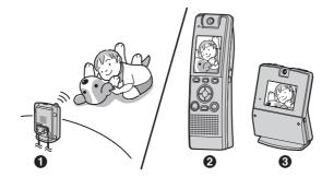
This feature allows you to view the room where the cordless camera ( $\textcircled{\bullet}$ ) is located from the units (O, O). You can also view the room between the units (O, O).
