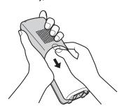
2 Insert the battery (1), and press it down until it snaps into position (2). Then close the handset cover (3, 4).
