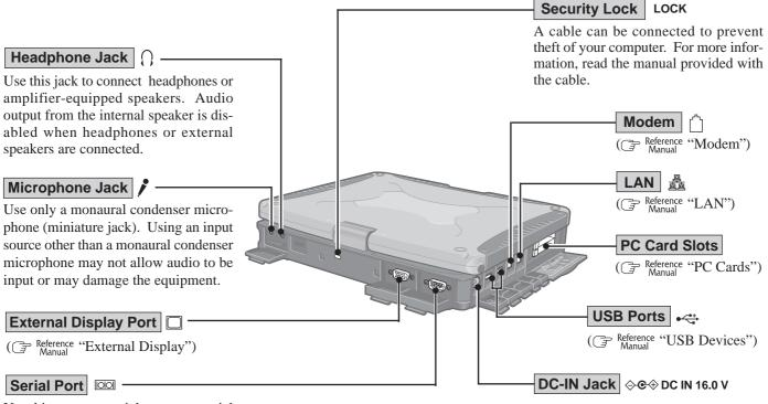
Use this port to a serial mouse or serial communication devices.
