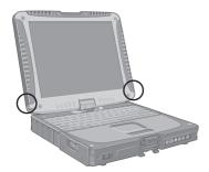
The tether can be attached to the bottom right or bottom left corner of the display. It prevents the stylus (included) from falling accidentally.
