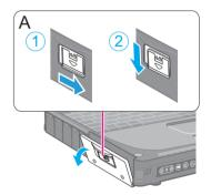
Insert the SD Memory Card with the label side facing up and with the cut corner facing in.
