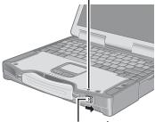
(3) Slide the battery pack inward until it is firmly in place.
