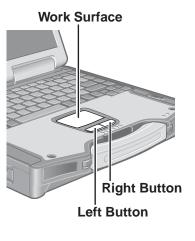
Use the touch pad to move the cursor on the screen and perform computer operations. For instructions on how to operate, refer to Reference "Touch Pad".
