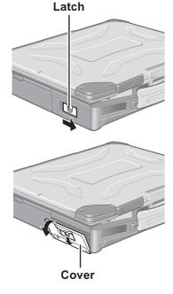
② Slide the latch down, and then without releasing it, open the cover as illustrated.
