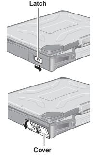
(2) Slide the latch down, and then without releasing it, open the cover as illustrated.
