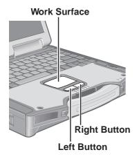
Use the touch pad to move the cursor on the screen and perform computer operations. For instructions on how to operate, refer to Reference "Touch Pad".
