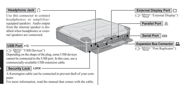
an input source other than a monaural condenser microphone may not allow audio to be input or may damage the equipment.
