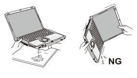
Keeping the computer level, move the computer to a dry place. If the computer is placed back on the wet surface, water may seep inside the computer from the bottom.
