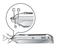
To store the stylus, push the end into (C). Push in the stylus so that the part (b) is aligned with (D).
