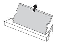
2 Gently remove the RAM module from the slot.
