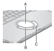
Use the touch pad to move the cursor on the screen and perform computer operations.
