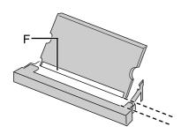
② Place the RAM module lightly in parallel with a slot. (The gold terminals (F) are visible)
