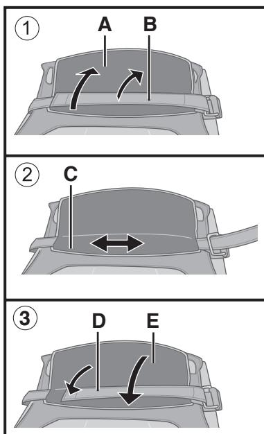
Adjust the fastening strength of hand strap as below.
