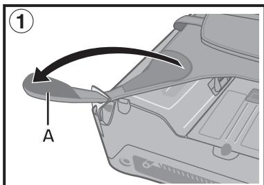
① Remove the edge (A) of hand strap passing through the clip. (The illustration shows the left side of hand strap as an example.)
