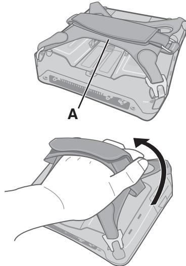
When using the computer holding with hand, insert your hand to (A) part of the hand strap. Fix the hand strap firmly so that the computer does not come off, and then turn it over.
