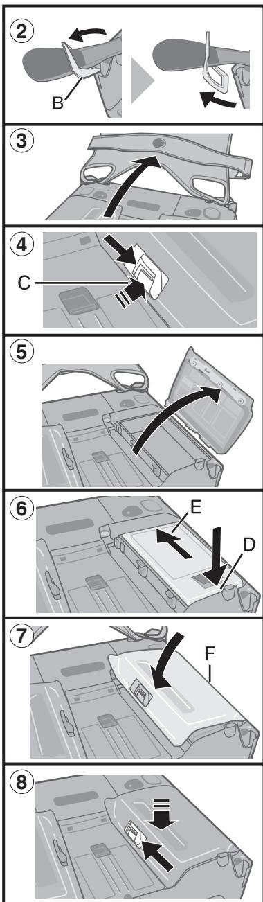
② Tip the clip (B) front to pull it out of the computer. (Do the same for the right side of hand strap.)
