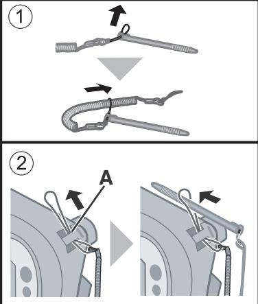
The stylus has already been attached to the computer at the time of purchase. Use the computer with the stylus attached not to lose it. If the stylus is removed for its position change or replacement, attach it according to the instruction below.
