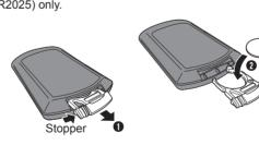
While pressing the stopper, pull out the battery
