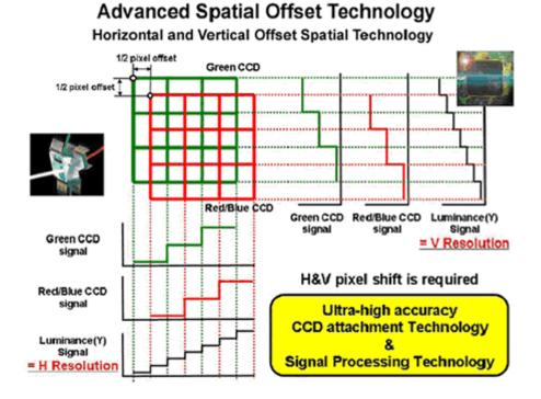
The optical block for this professional DVCPRO HD camcorder is assembled using highly accurate, patented technology to precisely set the Horizontal and Vertical pixel shift to ½ pixel. This gives the advantage of better dynamic range and sensitivity with minimal compromise in resolution.
