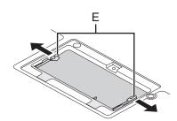
2 Carefully remove the RAM module from the slot.
