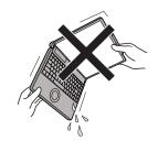
4 Keeping the computer level, move the computer to a dry place.
