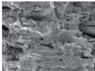
Random polymer orientation in metallic mold of a conventional mica-polypropylene cone.
