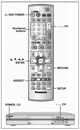
After plugging the unit into your household AC outlet and pressing [ტ, DVD POWER] to turn the unit on for the first time, the unit assists you to set the menu language, and automatically tunes in all the channels it can receive and sets the clock.
