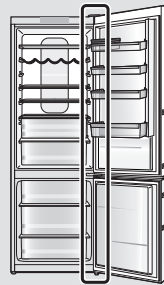
Potential pinch point
