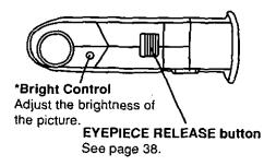
\*Note: This control has been set at the factory. It is not necessary to adjust this control under normal circumstances. But, should it become necessary, be careful to make the adjustment with a small, slender screwdriver so as not to damage the miniature control.
