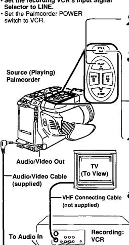
■ Insert a pre-recorded tape into the Palmcorder and a blank tape with a recording tab into your VĊR.
