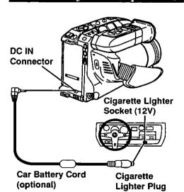
Connect a PV-C16 Car Battery Cord (optional) to DC IN on the Palmcorder.
