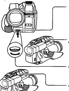
Press MANUAL FOCUS so that "MF" (Manual Focus) appears in the EVF.
