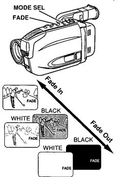
If FADE is accidentally pressed, simply press it again so that "FADE" disappears in the EVF.
