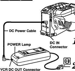
Connect VCR DC OUT on the AC Adaptor to DC IN on the Palmcorder with the DC Power Cable (supplied).
