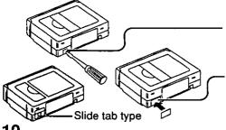
To prevent accidental erasure, break off the tab with a screwdriver. (If slide type, slide tab open.)
