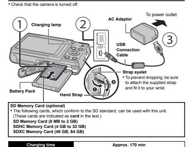
. When charging is complete, the charging lamp will go off - then you may disconnect the camera from the power outlet or compute
