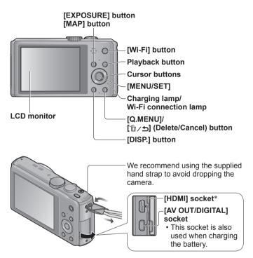
\* Do not connect any other cables except the HDMI micro cable (RP-CHEU15: optional). Doing so may cause malfunction.
