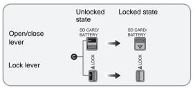
• Lock securely to the points where the red portion **O** of the open/close lever and LOCK lever are no longer visible.
