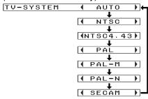
This should normally be set to "AUTO". If the signal is of such poor quality that the correct format cannot be automatically distinguished, change the setting manually to the required TV system.
