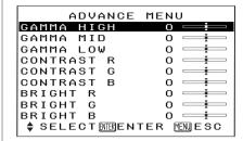
"GAMMA HIGH/MID/LOW" is used for correcting the gradation of a bright or dark projected image.
