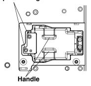
④ Insert the new lamp unit while making sure that the direction of insertion is correct, and then use a Phillips screwdriver to securely tighten the lamp unit fixing screws.
