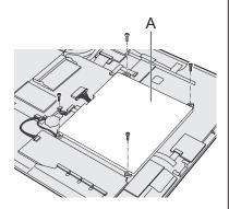
6. Disconnect the connector, and remove the built-in battery.
