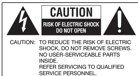
The lightning flash with arrowhead symbol, within an equilateral triangle, is intended to alert the user to the presence of uninsulated "dangerous voltage" within the product's enclosure that may be of sufficient magnitude to constitute a risk of electric shock to persons.
