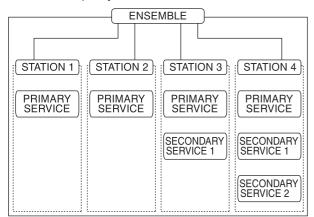
As shown in the diagram, an ensemble consists of a group of stations with primary services and secondary services. This means, for example, that commentary on sports events from different areas can all be broadcast at once.
