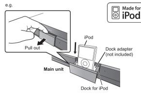
Attach the dock adapter which should be supplied with your iPod to the dock for the stable use of the iPod.
