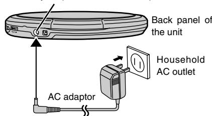
Recharging starts. The main unit's recharging lamp (CHG) lights and the battery indicator on the remote control scrolls.
