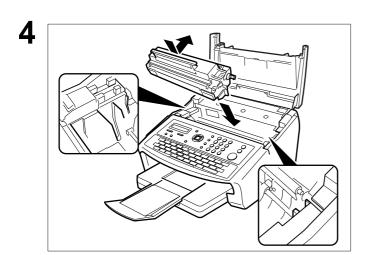
Align the projections on both sides of the Toner Cartridge with the grooves in the machine as shown and insert the Toner Cartridge into the machine.
