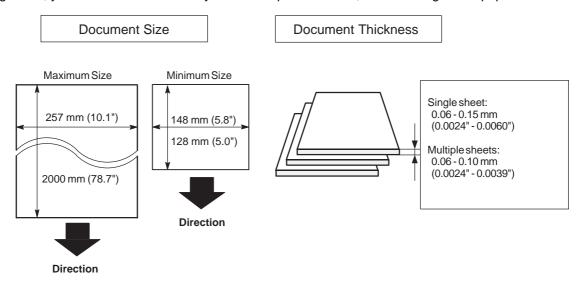
**Note:** The maximum document width that can be sent through the machine is 257mm (10.1"). However, the effective scanning width is 212mm (8.3").
