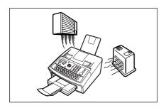
Do not place the machine near heaters or volatile, flammable, or combustible materials such as curtains that may catch fire.
