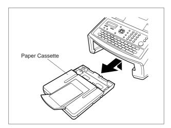
Lift up the Paper Cassette slightly and slide it out of the machine.
