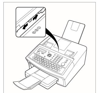
Slide the Pressure Adjusting Lever to the desired position depending on the condition.
