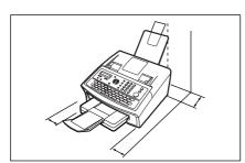
Install the machine on a flat surface, leave at least 10 cm (4") of space between the machine and other objects.
