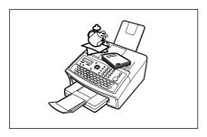
Do not place any heavy object on the machine. An off-balance machine can tip-over or the heavy object can fall, causing damage and/or injuries.
