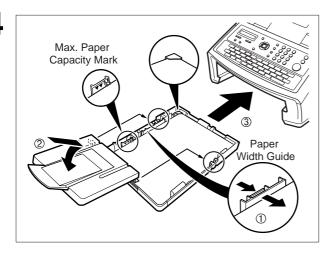
Load the paper into the Paper Cassette. Slide the paper width guide to the left until it lightly touches the stack of paper without bending the paper. The paper must fit squarely and firmly between the Paper Width Guide and the right side of tray. If it does not, the paper may feed into the printer incorrectly resulting in a paper jam.
