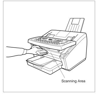
Wipe the Scanning Area gently with a soft cloth gauze moistened with ethyl alcohol. Be sure to use a clean cloth as the scanning area can be easily scratched.
