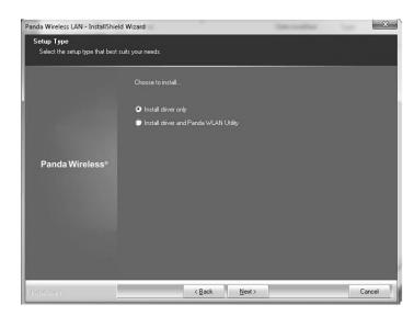
Note: Select "Install driver and WLAN Utility" if you want to set up your computer as a WiFi Hotspot/WiFi repeater with the Panda adapter.
