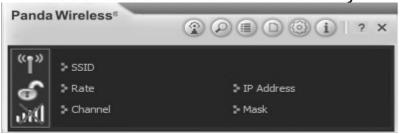
The Wireless Utility includes "AP Setup", "Available Networks", "Link Info", "Profile Settings", "Advanced", "About" and "Help" buttons in the upper right hand corner.
