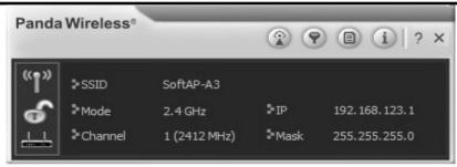
The Wireless Utility includes "AP Setup", "Access Control List", "Connected Devices", "About" and "Help" buttons in the upper right hand corner. Click the "AP Setup" button to create a new wireless network.
